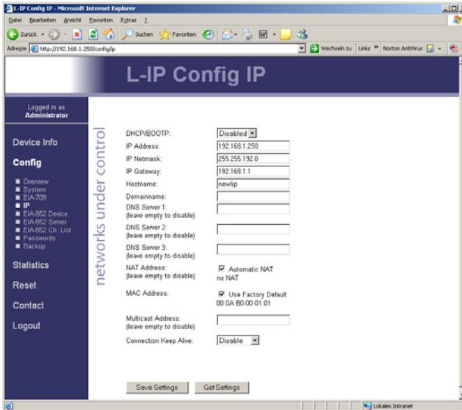
Press „Save Settings“ and then reset the device by selecting „reset“ in the highlighted text. This changes the IP settings of the CG-S / IP-router.
