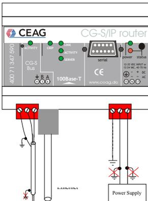
The CG-S / IP-Router enclosure is 6 TE (1 TE = 17.5mm) wide for DIN rail mounting following DIN 43 880:
